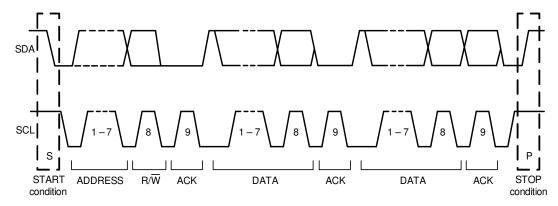
Figure 11: Complete I<sup>2</sup>C Data Transfer
