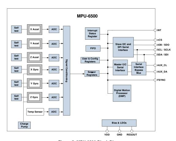
Figure 5: MPU-6500 Block Diagram
