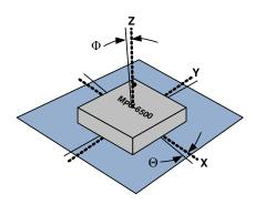
Package Gyro & Accel Axes (--- )Relative to PCB Axes ( —— )with Orientation Errors (Θ and Φ)
