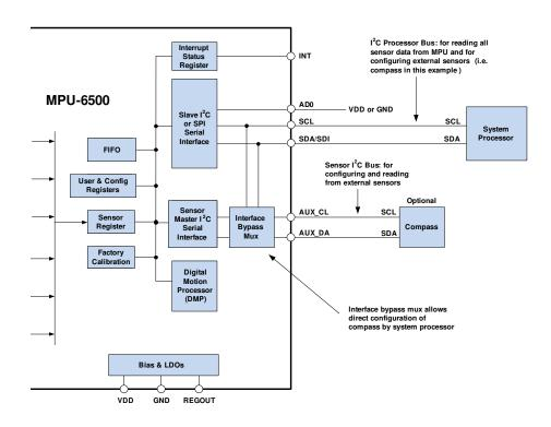
Figure 6: MPU-6500 Solution Using I<sup>2</sup>C Interface
