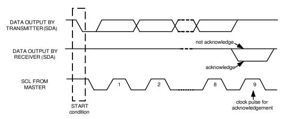
Figure 10: Acknowledge on the I<sup>2</sup>C Bus
