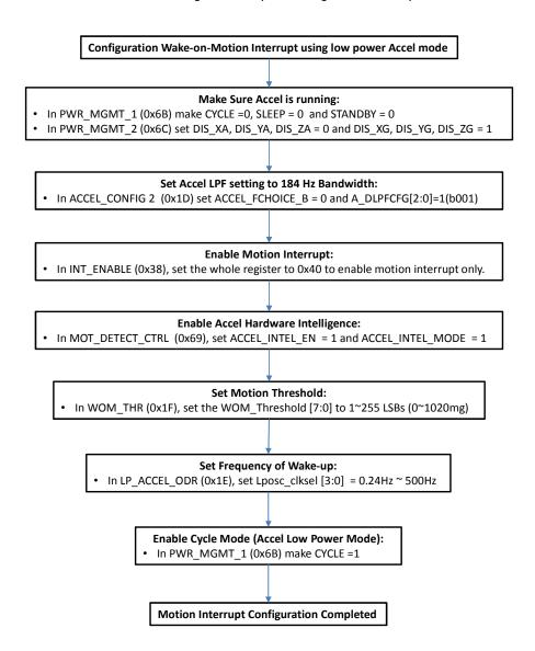
Figure 8: Wake-on-Motion Interrupt Configuration
