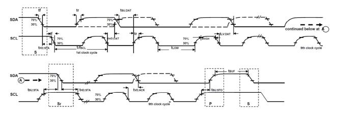
Figure 1: I2C Bus Timing Diagram
