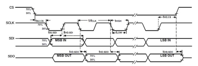
Figure 2: SPI Bus Timing Diagram
