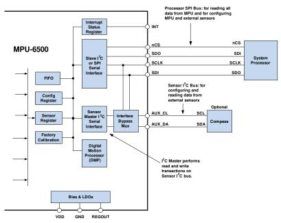
Figure 7: MPU-6500 Solution Using SPI Interface
