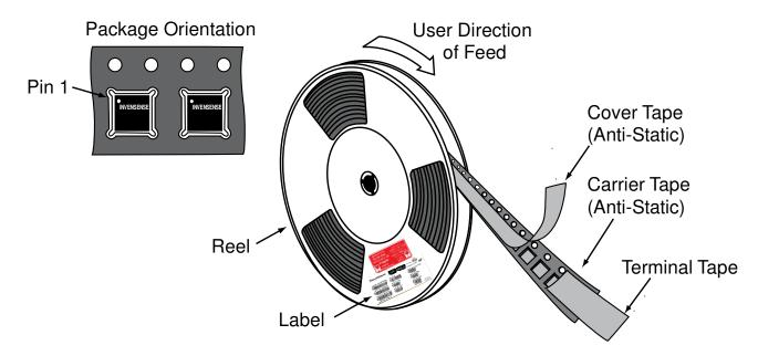
**Tape and Reel Specification – Package Orientation**
