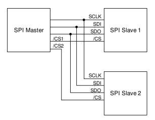
Figure 12 Typical SPI Master / Slave Configuration
