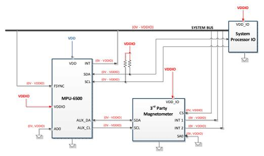
Figure 13: I/O Levels and Connections
