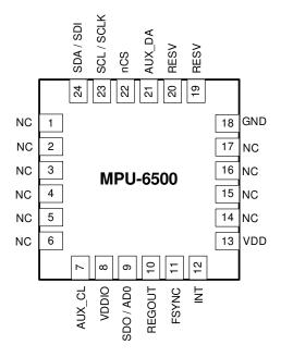
Figure 3: Pin out Diagram for MPU-6500 3.0x3.0x0.9mm QFN
