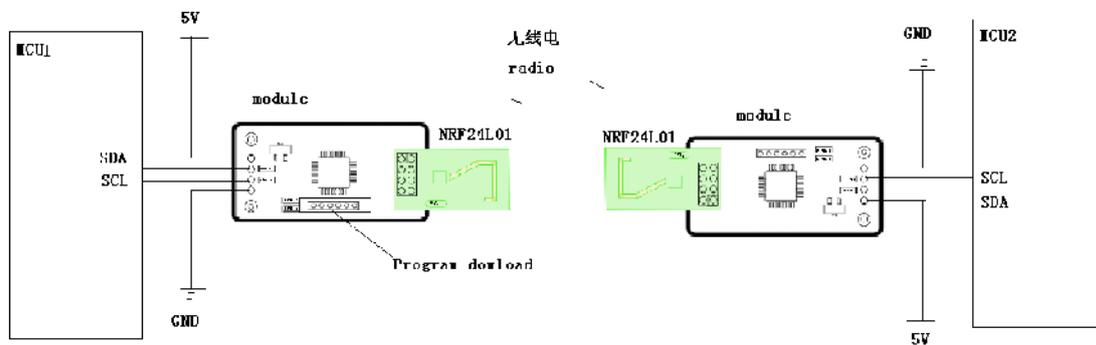
This module is used I2C/TWI communication, NRF wireless communication module used, it is safe and reliable. And it reduces the possibility of data lost greatly. In the communication process there are three stages: MCU reading data, Free Mode (MCU write data or NRF24L01 write data), Module busy mode(module sends data).
