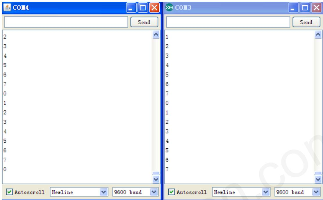
Description: This experiment is like this: Aduino ADK sends a data first , and then waits to receive the same data, if it has received data, then it will show the data as above picture COM3; Arduino UNO waits to receive data first, and then it will display the data after it receives every time, after that it will send back the data to module. So On Ad Inifinitum.
