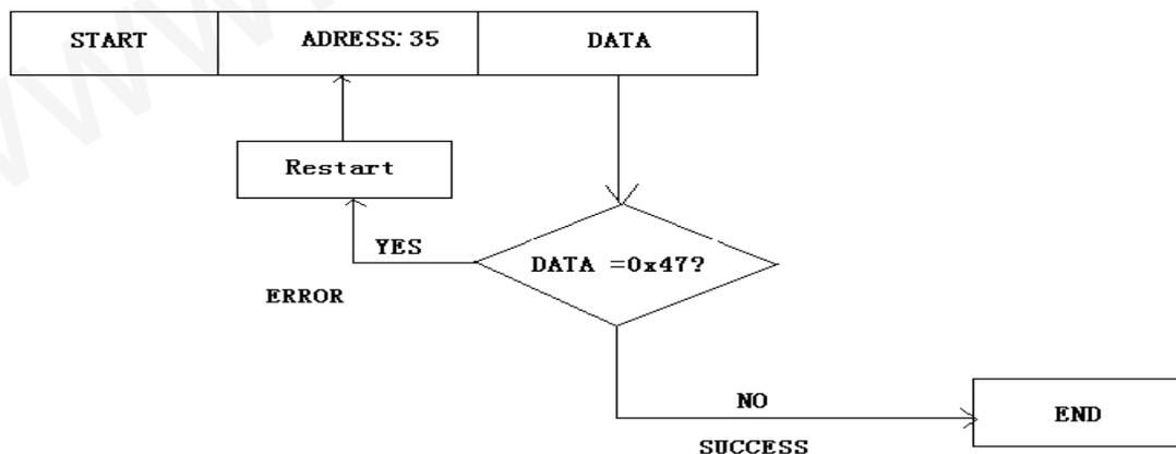
First MCU sends address to module, and module will response a signal if returned data is not "0x47", it indicates that reading data is successful.
