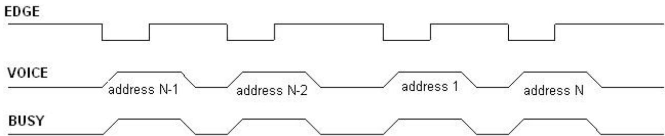
Remark: Edge trigger. One key trigger to play. A negative edge trigger a group of voice, next negative edge trigger previous group of voice, after finish first group loop to last group.
