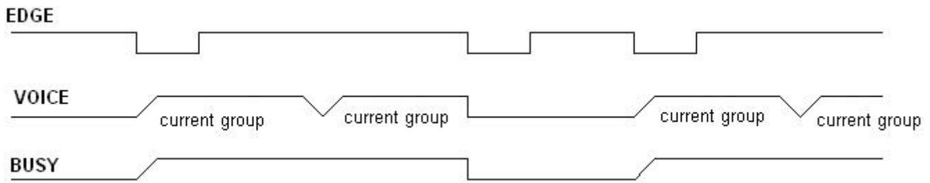
Remark: Edge trigger. When I/O test falling edge( such as this I/O short touch GND) ,the voice will be triggered. After play finished, will cycle play. During the playing , the next falling edge will stop the voice ,other falling edge will make it play again
