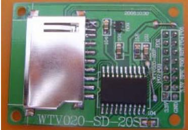
A green PCB with a silver metal SD card socket. A white plastic component is mounted above the socket. The text "WTV020-SD-20S" is printed at the bottom of the PCB. Various electronic components and a small orange capacitor are visible. |
