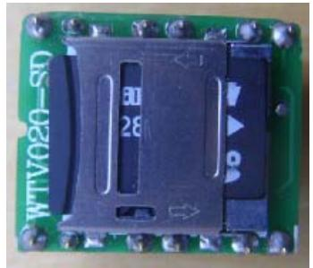
A green printed circuit board (PCB) featuring a black plastic SD card socket. The text "WTV020-SD" is printed vertically on the left side of the socket. The PCB has several pins along the bottom edge.                                      |
