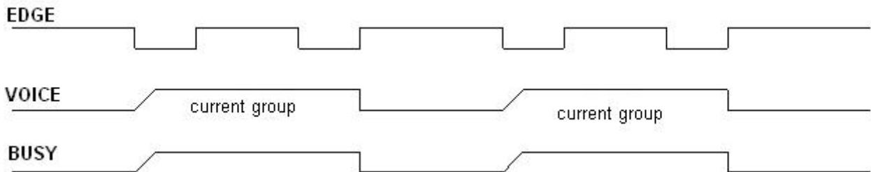
Remark: Edge trigger. A negative edge trigger to play, next negative edge to stop.
