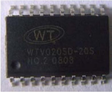
A black plastic integrated circuit (IC) package with a gold-plated metal lead frame. The package is marked with the letters "WT" in an oval logo, followed by "WTV020SD-20S", "NO.2 0803", and a series of numbers at the bottom.           |
